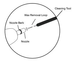
When cleaning, do not force any object through the earphone nozzle! This will damage the earphone sound filter.
